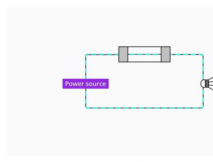
When this heating occurs, the metal alloyinside the fuse melts, causing the <u>power supply</u> to the direct to be interrupted. To work again, the fuse must be replaced, generating unnecessary labor, costs, and interruptions!
