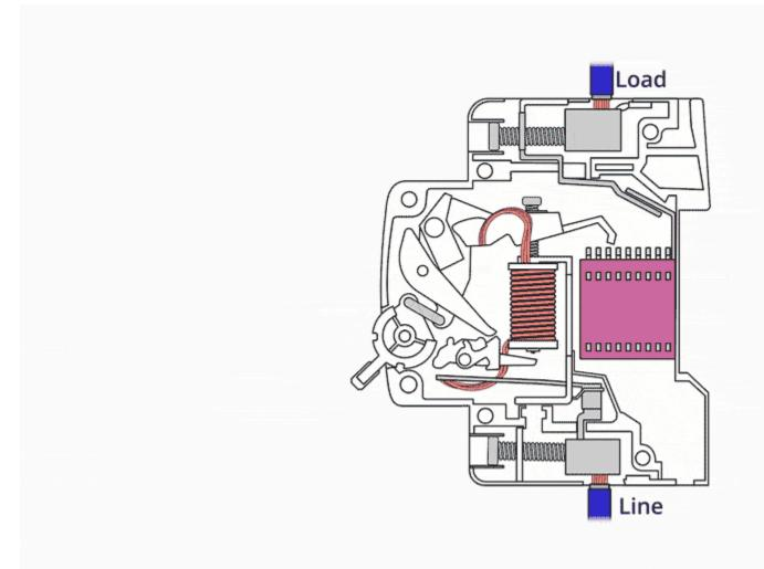
Differently from fuses, once the issues that caused the direct breaker to trip have been addressed, you can switch it back to the on position, and your direct is once again protected.
