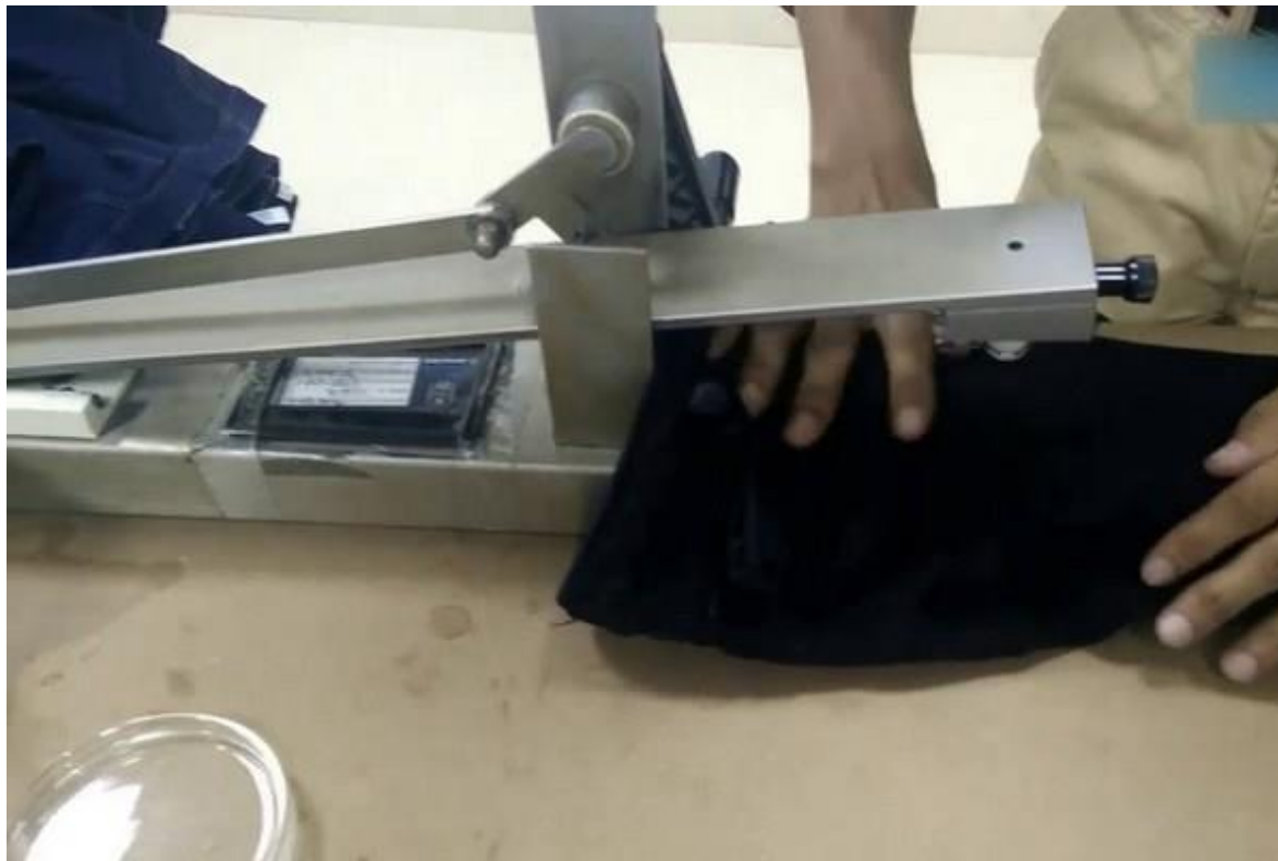
Figure 1: Rubbing fastness testing
