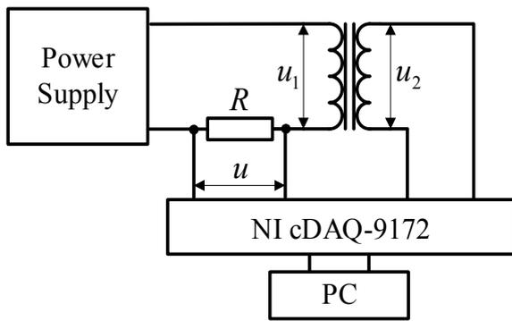
**Fig. 2.** Measurement setup based on personal computer
