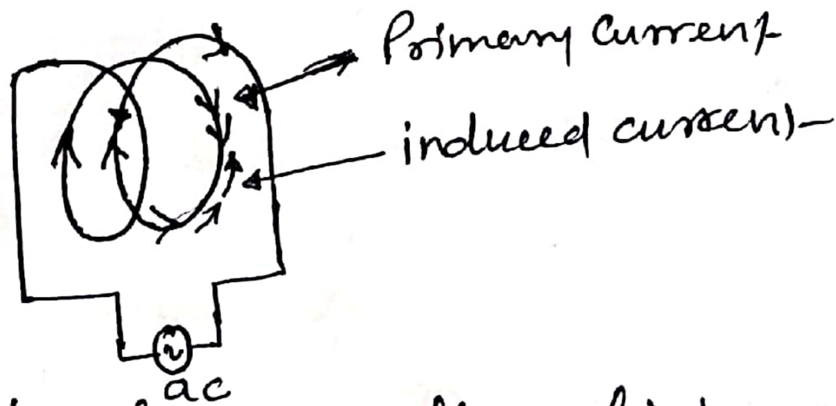
(III) Since time varying leakage flux links with the concerned winding itself, by electromagnetic induction it induces an emf (effect) through self induction in order to oppose the cause i.e. time varying current that created leakage flux.
