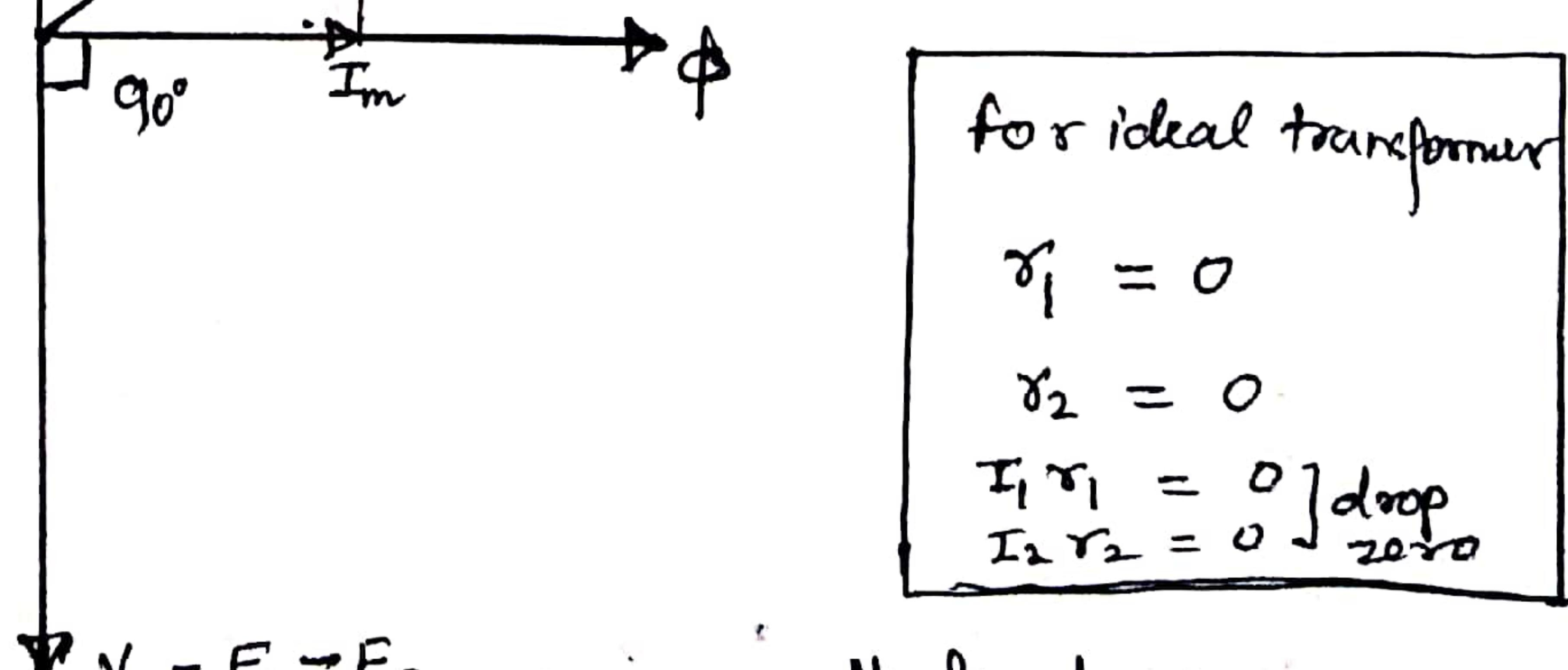
No load means secondary terminal is open circuited.
