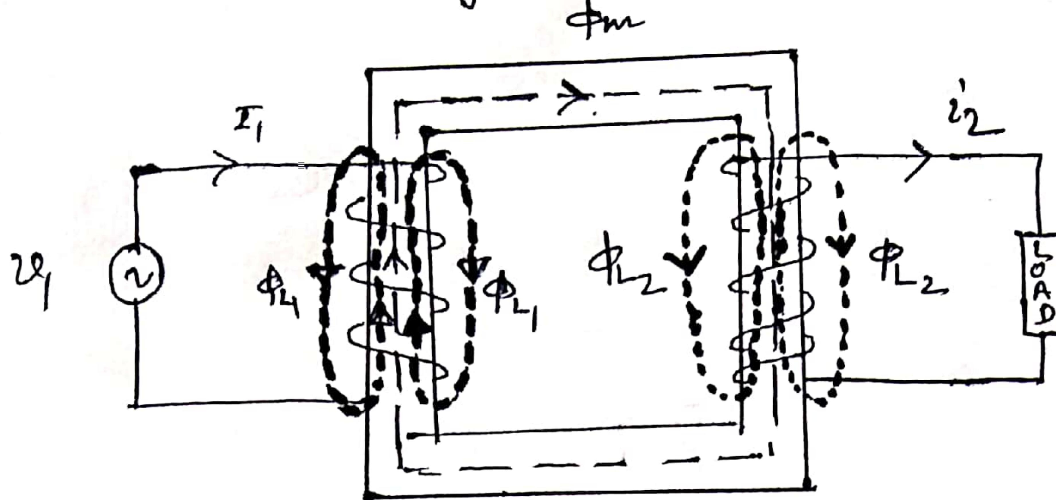
(I) Part of the total flux of a winding that links only with the winding itself and/or metallic body parts of transformer such as tank wall, core clamps etc. is called leakage flux.
