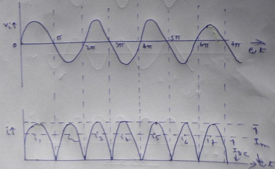
Under the action of sinusoidal AC voltage applied to the primary of the transformer, the AC voltage across the secondary, which is applied to the point A and C of the network is given by
