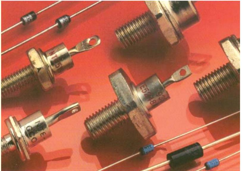
↑ A major application for zener diodes is voltage regulation in dc power supplies. Zener diode maintains a nearly constant dc voltage under the proper operating conditions.
