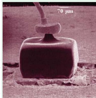
Discrete commercial Si tunnel diode
